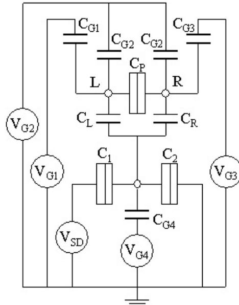
*Fig 2:* Simplified schematic circuit diagram of the device. Cross-capacitances have been omitted for clarity.
