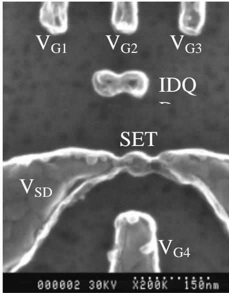
*Fig 1:* SEM micrograph of the fabricated device, with the isolated double dot capacitively coupled to a connected single dot.
