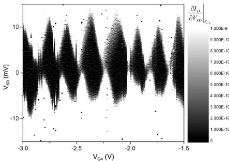
*Fig 3:* Differential current stability diagram of the single quantum dot electrometer at 4.2K. The device exhibits Coulomb blockade within the black regions. Each Coulomb diamond corresponds to the addition of an electron to the SET-island as  $V_{G4}$  becomes more positive.
